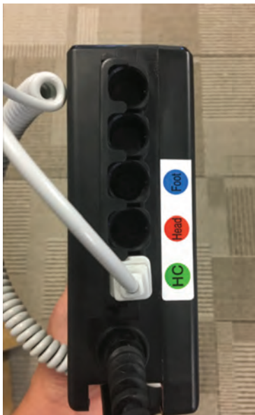
Figure 13: Junction Box, Semi-electric bed
