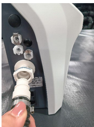
Attaching main air delivery line
