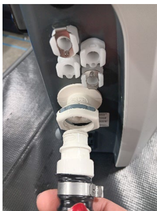
Attaching main air delivery line
