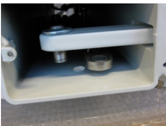
Picture 10: Detach the circlip on the opposite side by means of the circlip pliers, too.
