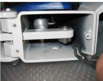
Picture 10: Detach the circlip on the opposite side by means of the circlip pliers, too.
