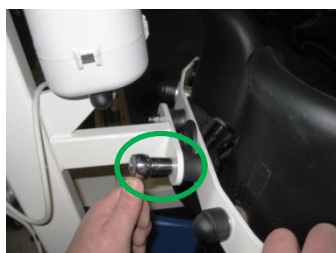
Picture 3: Loosen and detach the locking nut marked in the picture.
