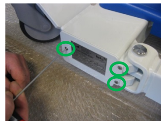
Picture 2: Detach the 3 screws marked in the picture.
