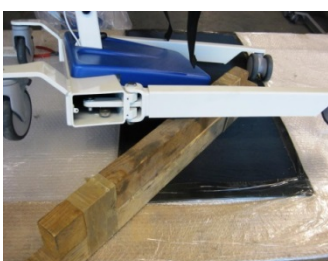
Picture 12: Mount an elevation (appr. 20 cm) under the chassis.
