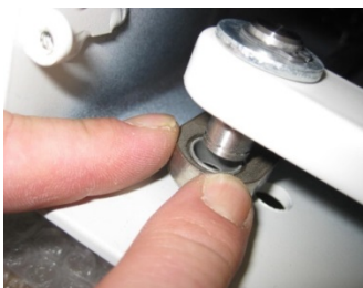
Picture 8: Detach the linkage from the guide bolt.
