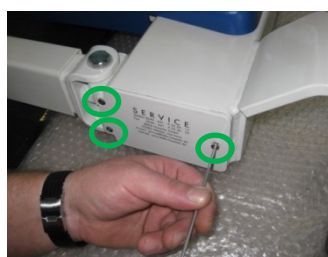
Picture 4: Detach the 3 screws marked in the picture.
