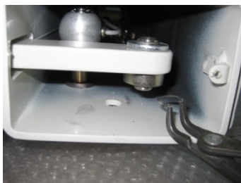
Picture 7: Detach the circlip by means of the circlip pliers.
