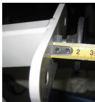
Picture 7: When mounting the new pressure piece, please observe the specified distance (2 cm). Lock the pressure piece by means of the counternut.
