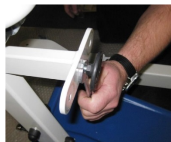
Picture 6: Loosen and detach the pressure piece.
