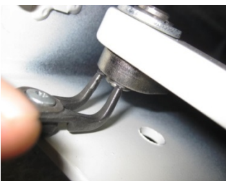
Picture 6: Set the circlip pliers to the circlip.
