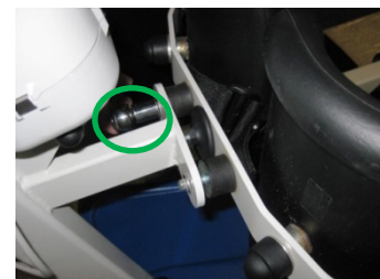
Picture 4: Loosen and detach the locking nut marked in the picture.
