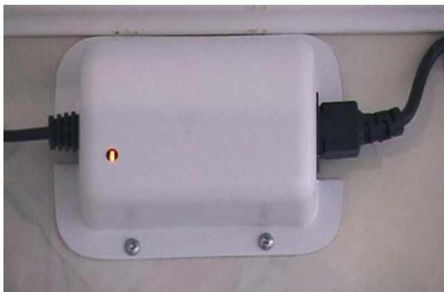
Charger with ORANGE light indicating that the lift is connected and charging. When the lift is fully charged this light will turn GREEN .
