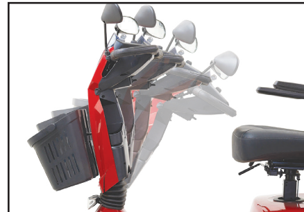
Infinite adjustable tiller with ergonomic design
