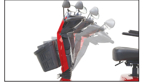
Infinite adjustable tiller with ergonomic design
