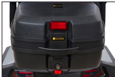
Lockable water-resistant storage compartment comes standard and attaches to the accessory bracket.
